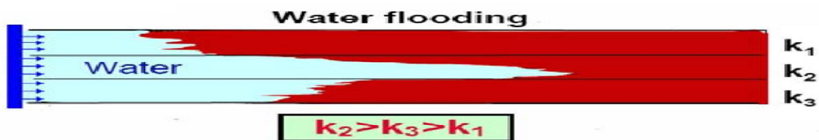
Fig. 2: Fingering of water into the oil bank for mobility ratios greater than 1
