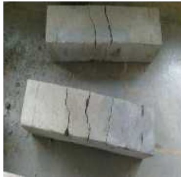
Fig. 7 Failed RCC Beam Specimens
