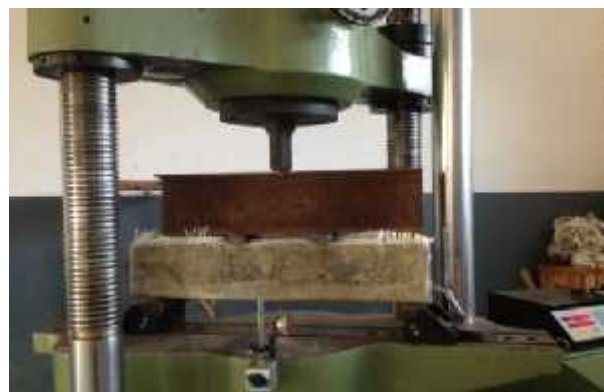
Fig. 8 Failed RC Beam wrapped with GFRP
